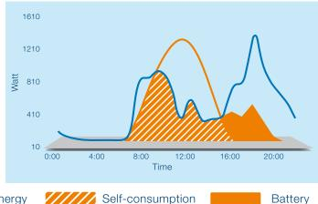
A photovoltaic system produces more energy in the middle hours of the day, but by contrast energy usage is greater in the evening hours.
